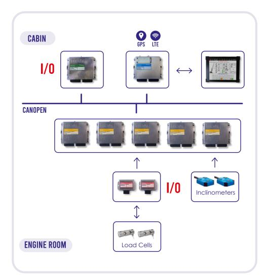
The master unit is the **DCU-C** combined with an external VGA touch-screen display, is also used as a human machine interface.
