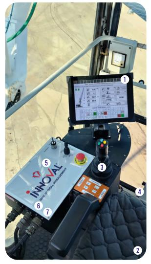
**1. Display** touch-screen VGA with integrated virtual keyboard
